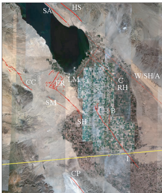
Figure 7. Known and inferred faults in the southern Salton Trough region. Most were taken from the Qfaults database ( http://earthquake.usgs.gov/regional/qfaults/ , last accessed July 2008). SA denotes San Andreas, HS denotes Hot Springs, CC denotes Coyote Creek, ER denotes Elmore Ranch, C denotes Calipatria, RH denotes Red Hill, W/SH/A denotes Wister/Sand Hills/Algodones, SM denotes Superstition Mountain, SH denotes Superstition Hills, B denotes Brawley, I denotes Imperial, CP denotes Cerro Prieto. LM is the fault inferred by Lohman and McGuire (2007) from the 2005 earthquake swarm. The Calipatria and Red Hill faults locations were taken from Figure 5.
